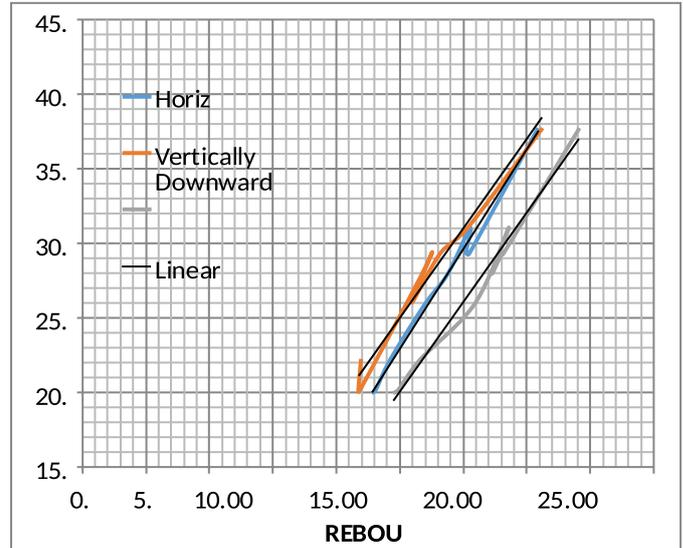
Fig. 3.2: Calibration curve for Rebound hammer
