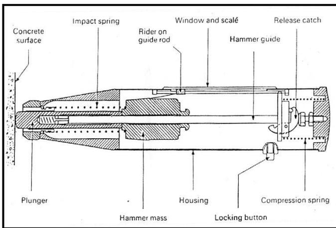
Fig 3.1: Components of Rebound hammer test
