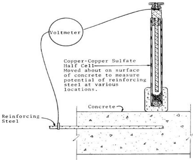
**Fig. 3.3:** Procedure for Half-cell Potential Test
